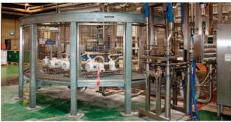
gallon drums. Fenney describes the concept as based on a semi-circle configuration feeding six stations, with each station able to datum a pallet holding the drums.
